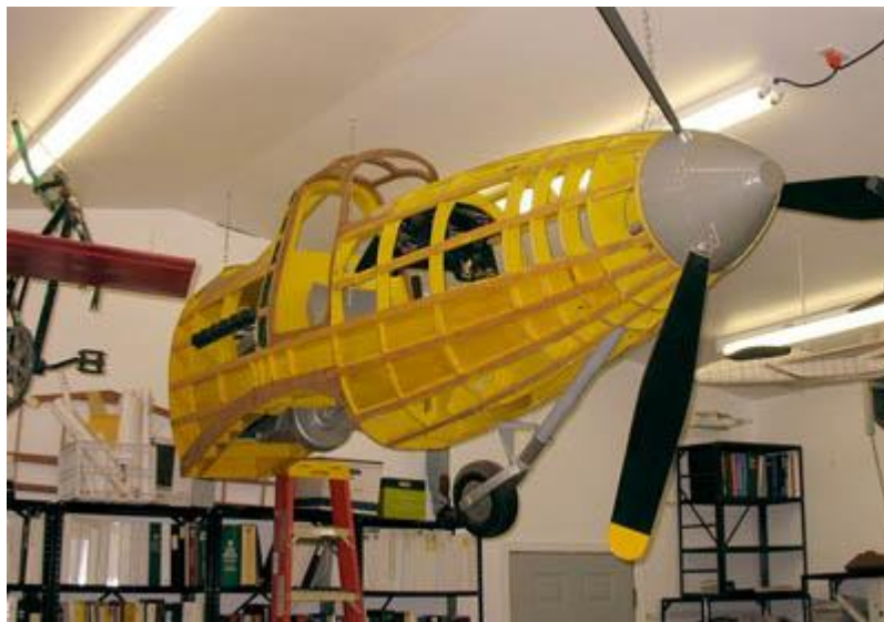
70 percent P-39 cockpit and nosecone mock-up
