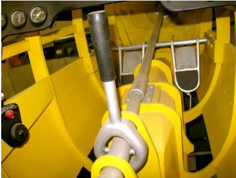
The driveshaft is seen running from behind the seat, through a carrier, and to the nose.
