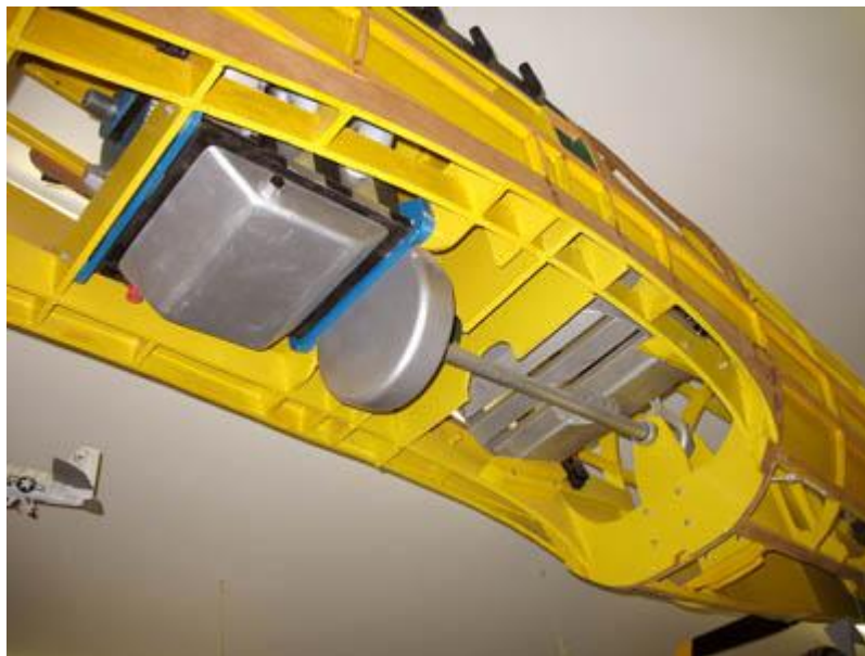
Mazda with PSRU and driveshaft
