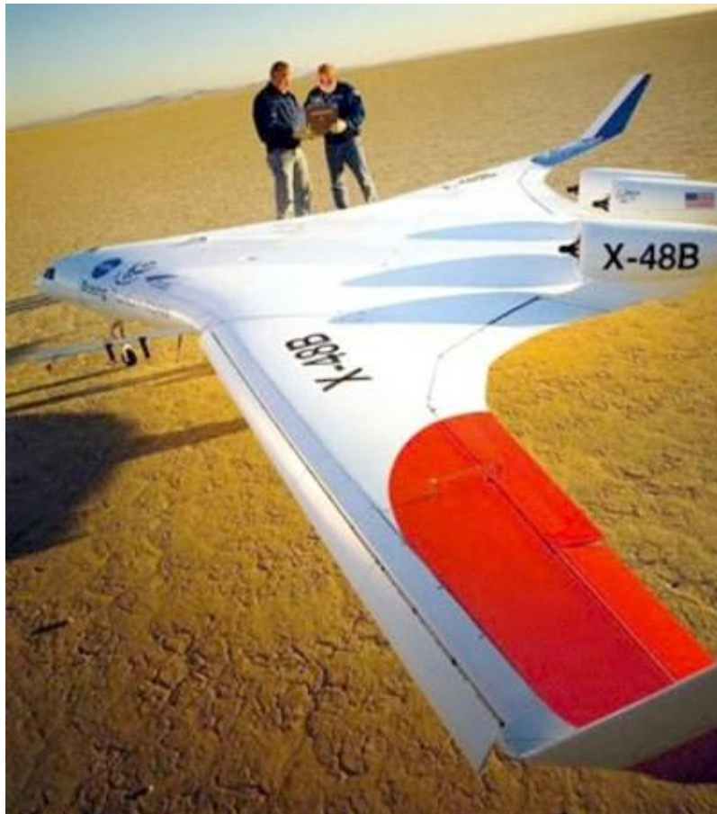
Boeing blended wing 8.5% scale R/C jet engines
