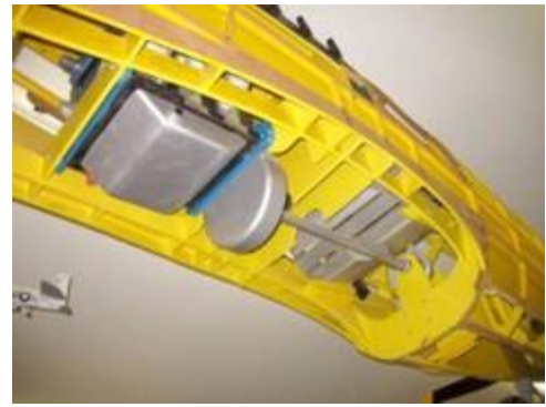
Photo 2, Mazda with PSRU and driveshaft
