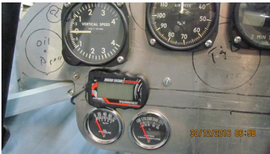
Tach Mounted on Panel with Velcro
