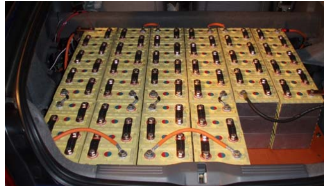
Figure 5 Battery pack in an electric car showing 64 of the 100 batteries in the pack
