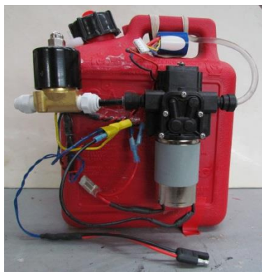
Assembled smoke tank with pump and solenoid valve
