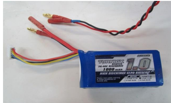
Lithium Battery, 1000 mah, 4s Held in place with a large elastic band for easy removal for charging (First version)
