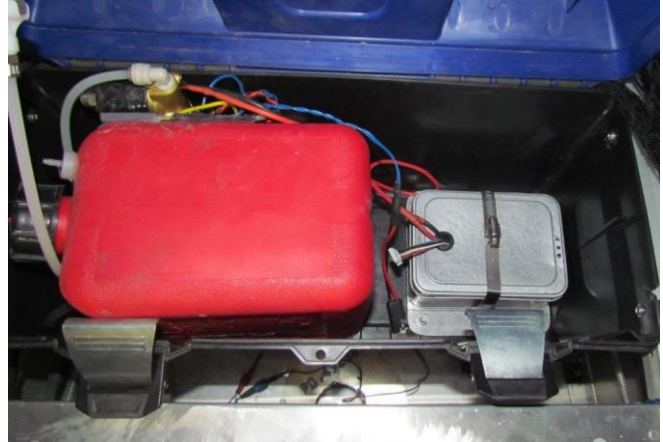
Smoke system installed in airplane.
