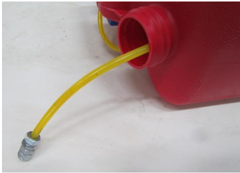
Inside end of the “Flop” tube The tube is glued into a 1/4” hole through the top of the fuel can. The inside end is weighted with (4) 1/4” stainless nuts
