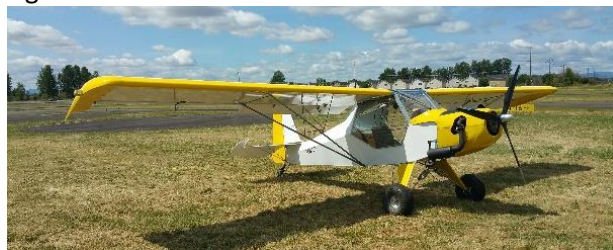
Patrick Hatfield Finished his Zenith CH-701 powered by a Rotax 912 engine.
