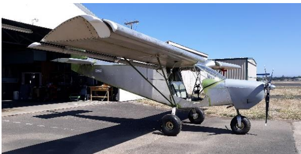
Patrick Hatfield Finished his Zenith CH-701 powered by a Rotax 912 engine.
